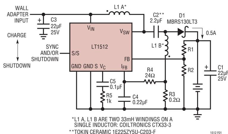
Figure 1. SEPIC Charger with 0.5A Output Current
