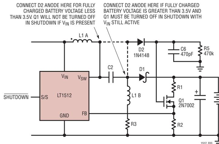
Figure 3. Eliminating Divider Current
