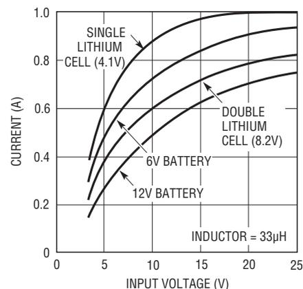
ACTUAL PROGRAMMED CHARGING CURRENT WILL BE INDEPENDENT OF INPUT VOLTAGE AND BATTERY VOLTAGE IF IT DOES NOT EXCEED THE VALUES SHOWN. THESE ARE ELECTRICAL LIMITATIONS BASED ON MAXIMUM SWITCH CURRENT. PACKAGE THERMAL LIMITATIONS MAY REDUCE MAXIMUM CHARGING CURRENT. SEE APPLICATIONS INFORMATION.
